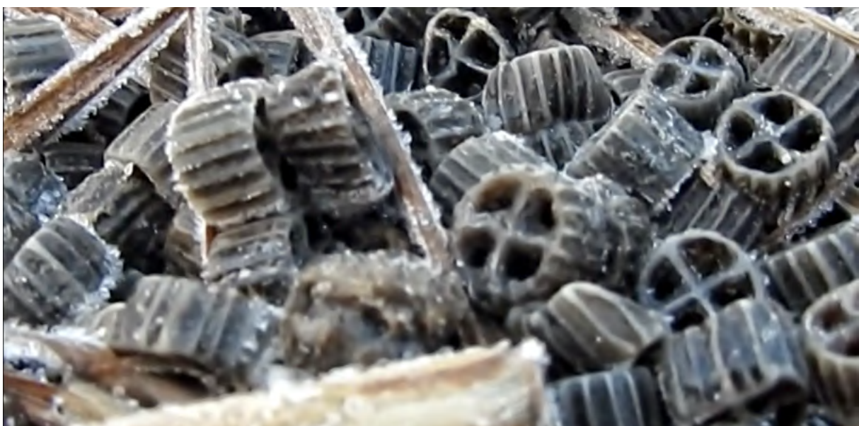
Figure 33 | Below | Biomedias type K1 collected on the shore after the incident at Nyköping WWTP, © Pontus Stenberg/SVT
